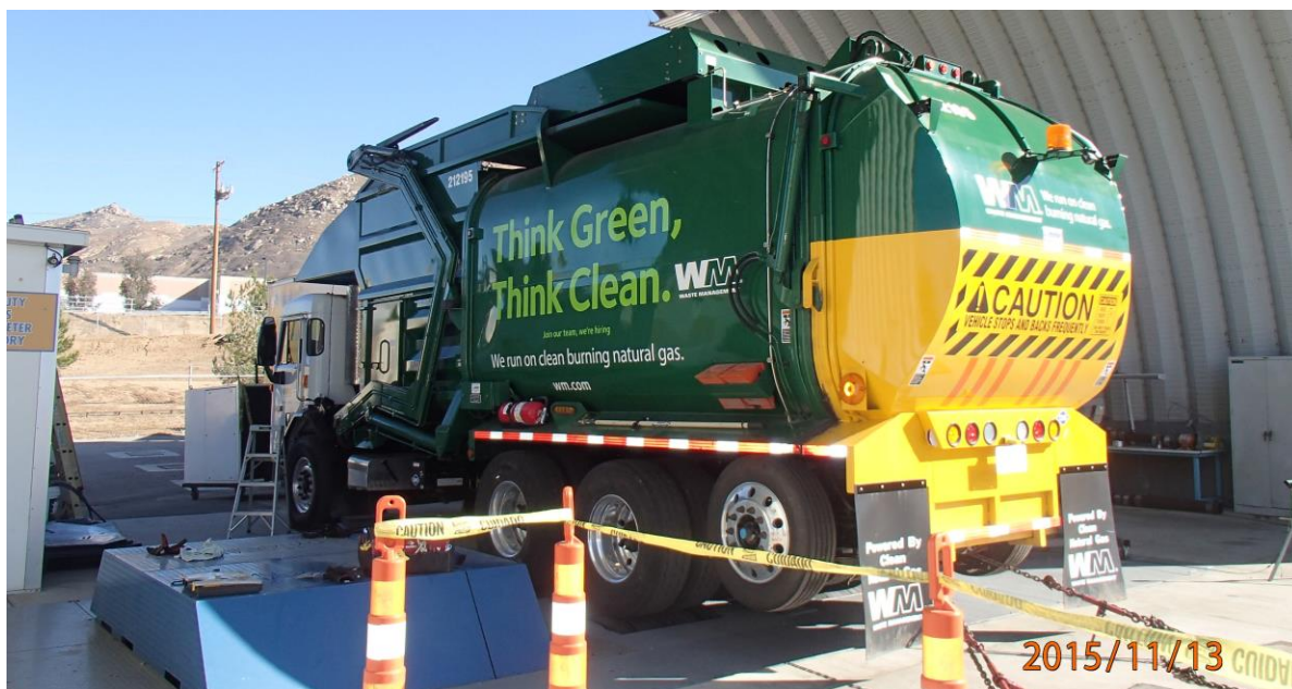
Figure 2-4 UCR's heavy duty chassis eddy current transient dynamometer
