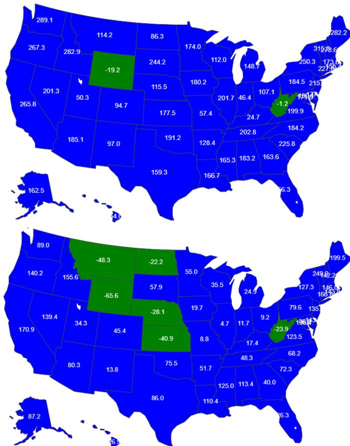
**Figure 2:** CO<sub>2</sub>eq emissions comparisons between a propane and an electric school bus using baseload (above) and non-baseload (below) emissions.
