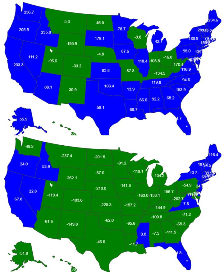
**Figure 3:** CO<sub>2</sub>eq emissions comparisons between a propane and an electric school bus using baseload (above) and non-baseload (below) emissions.
